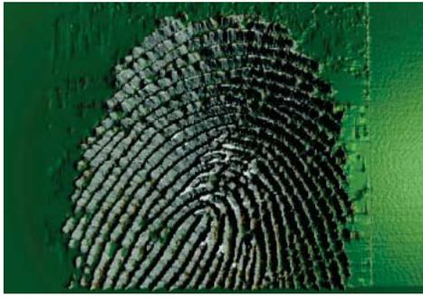
Figure 5. Scanning Kelvin Probe electrical potential data visualized as a three-dimensional surface relief map. Courtesy of the School of Engineering, University of Wales, Swansea.
